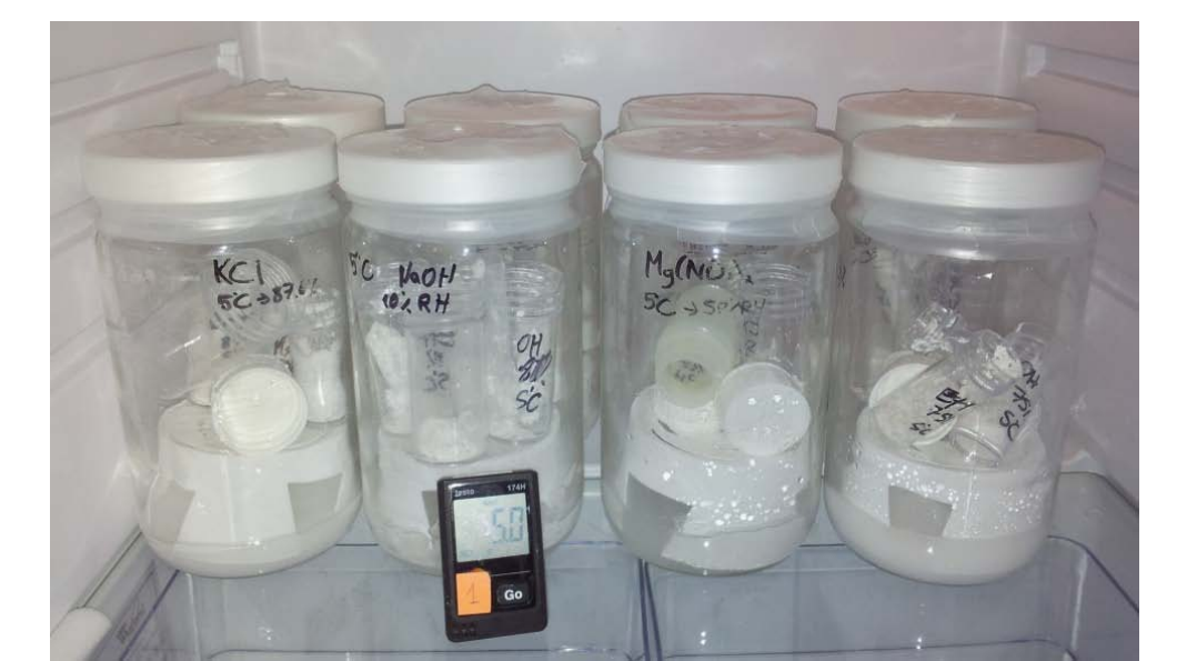
Fig. 2. Glass bottles equilibrated at 5°C and different RH with salt solutions. Pure synthetic samples are aged inside for several months before testing.
